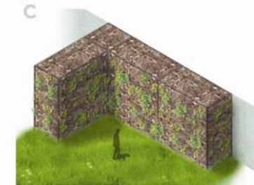
Gabions - Brick Fill with Planting
